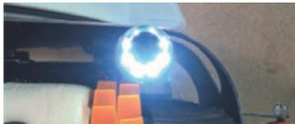
Waterproof IP68 camera with 8 LEDs
