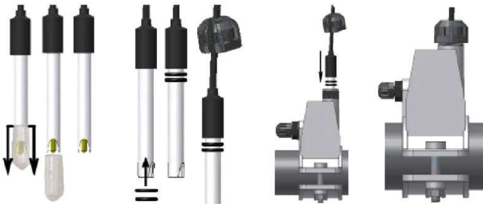
Fig. 3- Mounting the probe in the probe-holder
